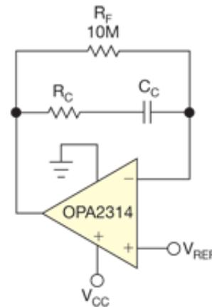
**Figure 9** Add series resistor  $R_C$  and capacitor  $C_C$  in the local feedback of the DRL amplifier.
