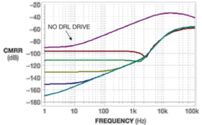
**Figure 4** Gain is higher in circuits with no DRL drive.
