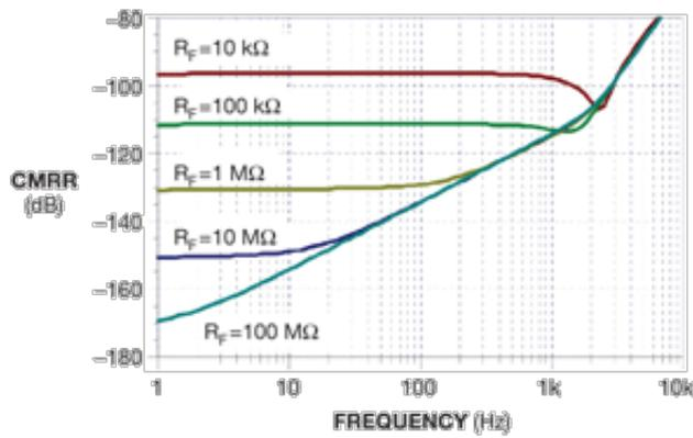
**Figure 3** Eliminating the dc path, setting  $R_F$  to a high value, or using both of these methods may be impractical for applications that require linear operation of the DRL amplifier when you remove one of the input amplifier leads.
