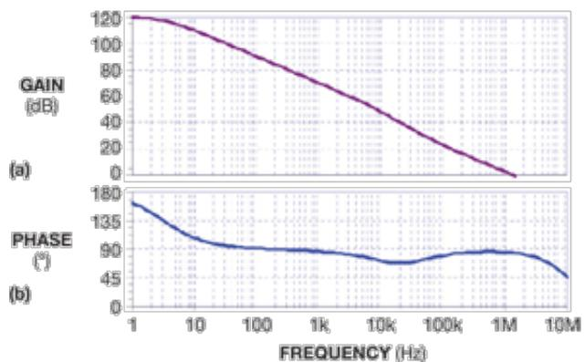
Figure 13 The overall beta curve intersects the open-loop-gain curve with a rate of closure that is 20 dB per decade or less and a loop gain (a) with a phase margin greater than  $45^\circ$  (b).
