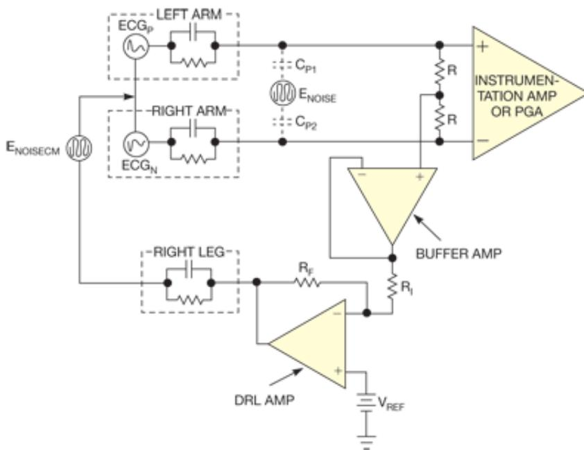
**Figure 1** The positive and the negative ECG sources, ECG<sub>P</sub> and ECG<sub>N</sub>, split to show how the DRL amplifier provides the common reference point for a portion of the ECG signal that the positive and negative inputs of the instrumentation amplifier sees.
